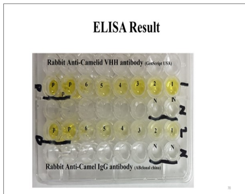
Figure S3. Result of ELISA test for VHH production of six colonies using two different antibodies
